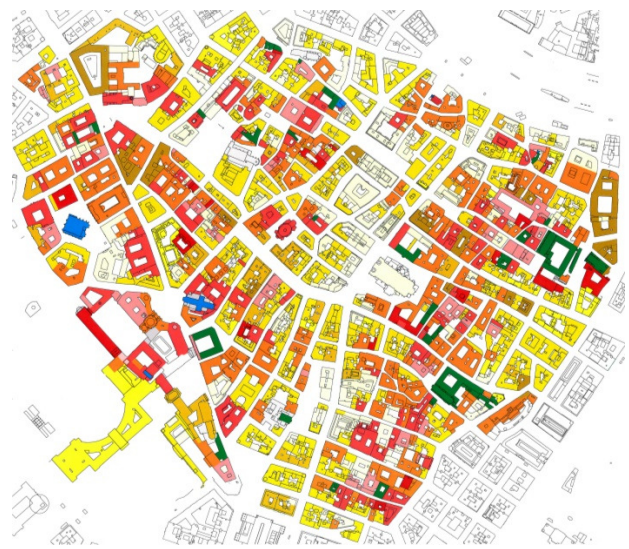
Figure 4: Provisional map of the roof structures in the historic city centre with building age (Blue - Gothic; Green - Renaissance; Red - Baroque; Orange - Classicist; Ochre - Gründerzeit; Yellow - 20 th century)
