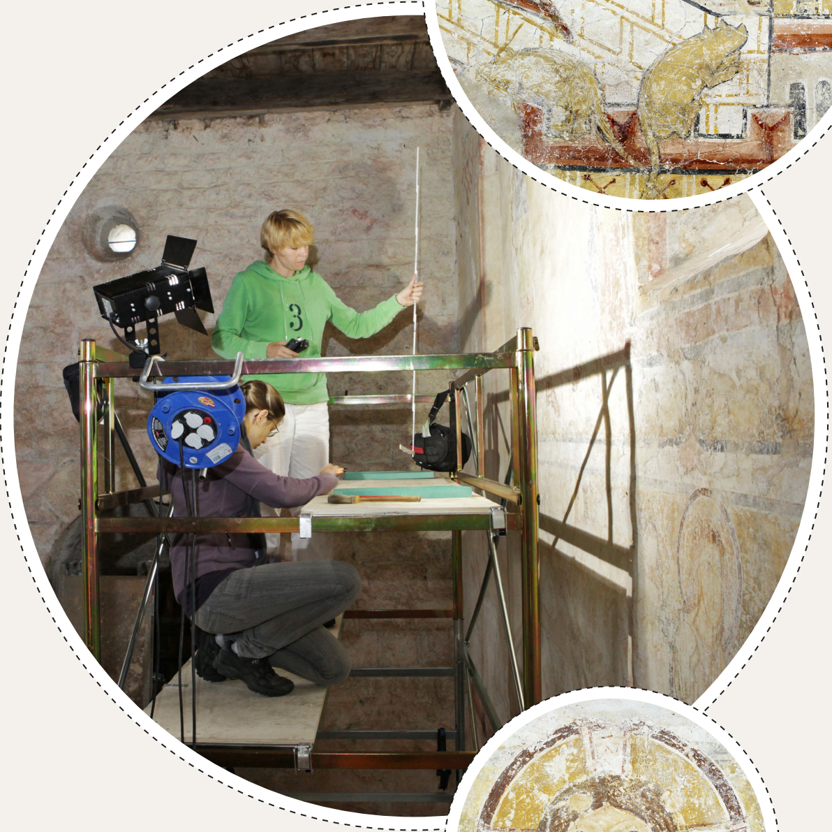
Measuring the surface conductivity on the Romanesque wall paintings in the St. John's Chapel in Pürgg
